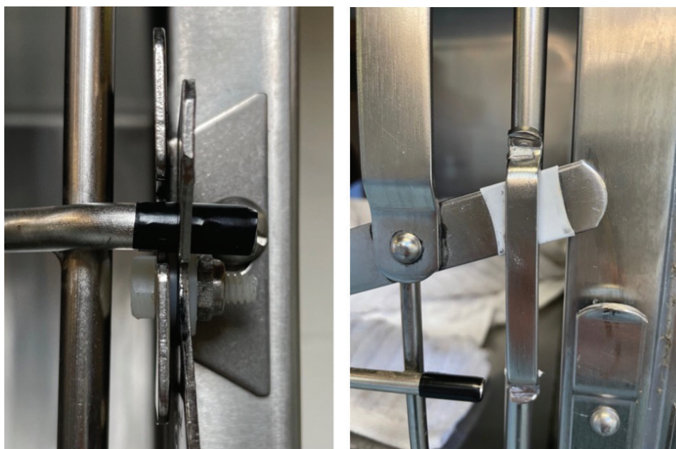
Fig. 2. Use of quiet latches or low-cost tape retrofits on cage latches can support noise mitigation and other low-stress care protocols.
